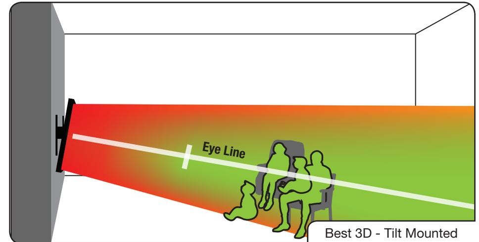
In this example, the viewers have mounted the TV on a **Tilt Mount**. They are at the correct distance and they are viewing the TV straight-on, close to the ideal eye line. They will experience good 3D picture quality.
